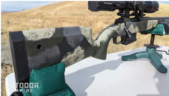
Generally speaking, carbon fiber stocks are lighter than synthetic plastic or polymer stocks, which are lighter than wood stocks.
