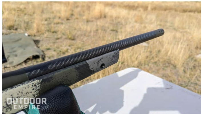
Carbon fiber wrapped barrels like this one on the Springfield 2020 Waypoint we tested help stiffen the thinner-than-usual steel barrel underneath.
